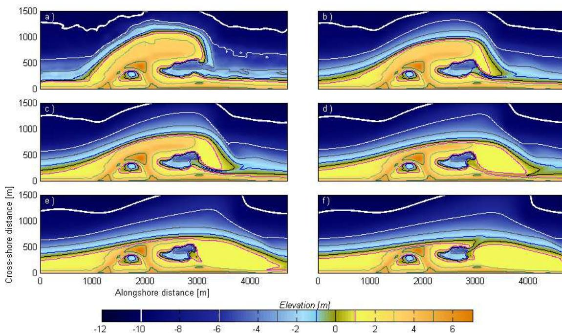
**Figure 4.** Long term model predictions of the morphological development of the Sand Engine. Panel a shows the initial model bathymetry, panels b–f show the prediction 3, 5, 10, 15 and 20 years after construction. Blue colors indicate sub-aqueous zones, yellow to brown colors show the sub-aerial beach and green colors indicate the intertidal area between high and low water. Depth values of the contour levels are indicated in the color bar (after Stive et al, 2013).
